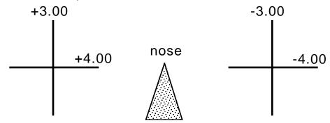
In the calculation we may ignore the prism contributed by the segments since that will be the same in both eyes. From Prentice's rule, then, the prism encountered one centimeter below the optical center of the right eye is (+3.00D)(1cm)=3p.d. BU. For the left eye it is (-3.00D)(1cm)=3p.d. BD. The prismatic imbalance is |+3-(-3)|=6p.c., a serious problem.
