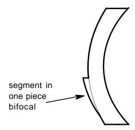
In one piece segments, cylinder is ground on the side of the lens opposite the add. Since minus cylinder lenses are standard today, this means the add is on the front of the lens.
