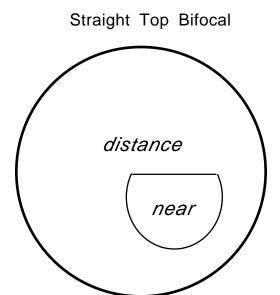
The straight top bifocal comes in a variety of shapes and sizes. Those commonly available today are the ST25, ST28, and ST35 which are 25mm, 28mm, and 35mm indiameter, respectively.
