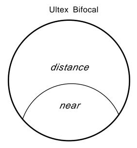
The Ultex bifocal is a round segment with a **very** big diameter. Unlike other bifocals, this one piece design is usually placed on the **back** of the spectacle lens.
