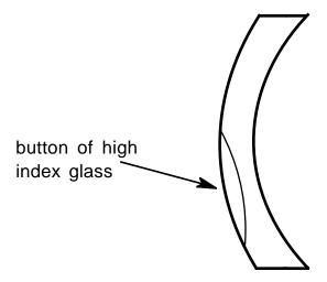
The curvature of the countersink curve can be calculated from paraxial optics knowing the add power, the front surface curve of the lens, and the indices of the two kinds of glass.
